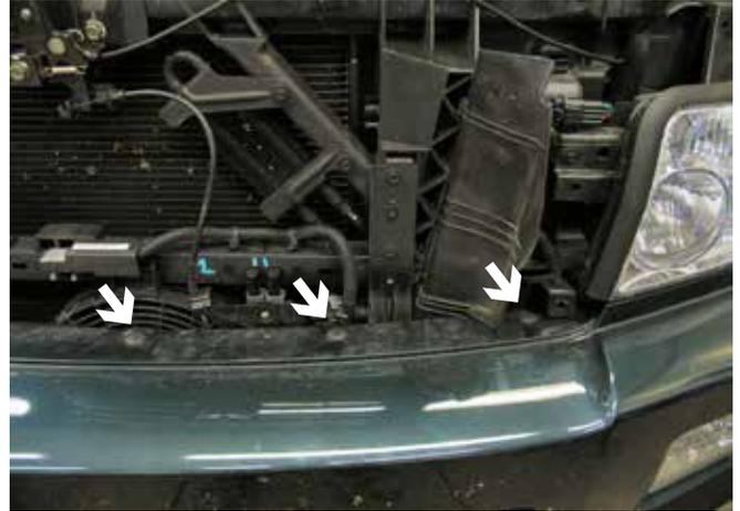
2. Remove 3 push pins from the front fascia on both sides of the vehicle. Just inside headlight assembly.
