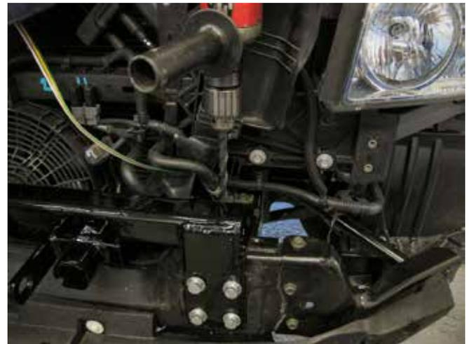
12. Align the baseplate with tow hook bolt locations. Finger tighten the 201-0153 hex bolts with lock washers. Slide 107-2681 between the top of the frame and back hole in baseplate. Tighten the 8-201-0153 hex bolts. Using the baseplate as a template, drill the back hole of the baseplate into the top of the frame with 17/32" drill bit, this will need to be done on both sides of the vehicle. Then install the last bolt.\*\*
