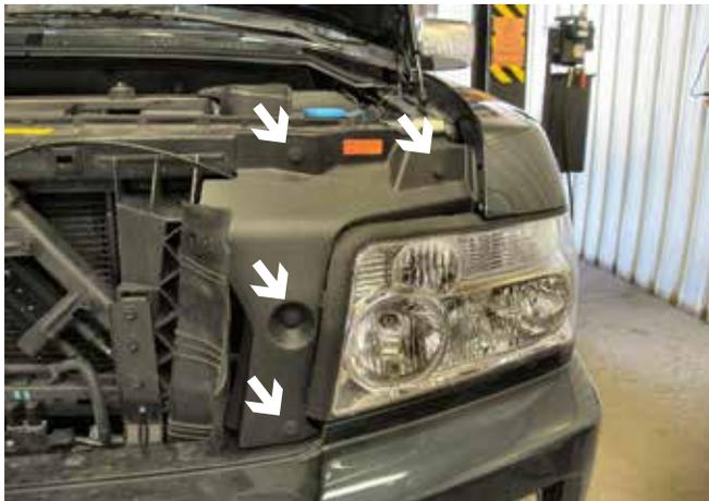
1. Remove 4 push pins from the front fascia near each headlight housing.
