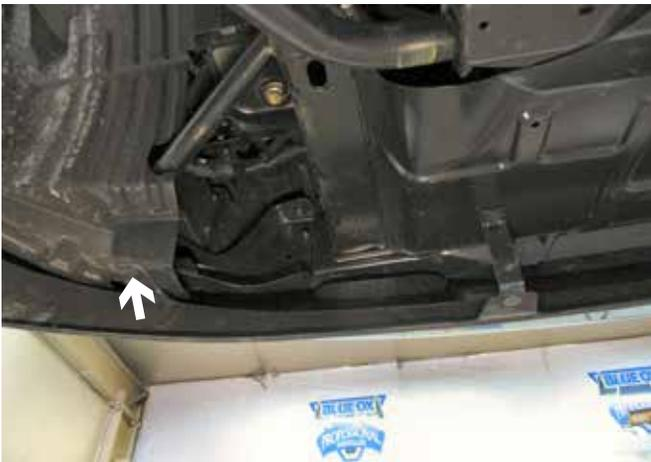
5. Using a 10MM Socket, remove 1 metric bolt and set aside. This is done on both sides. (The driver's side is shown).
