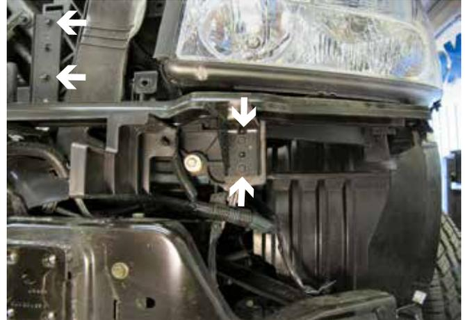
11. Remove 8 metric bolts with a 10MM Socket from the metal fascia support bracket, 4 metric bolts need to be removed from the hood latch. Which located right behind the metal fascia support bracket. Remove bolts from both sides. Pull forward on the bracket to remove it and set aside. (The driver's side is shown).\*\*
