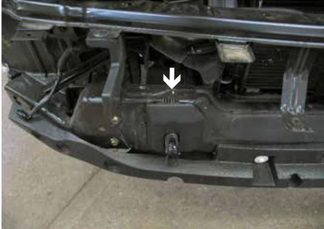
9. Remove push pin on top of where the tow hook attaches to the metal bumper. Take plastic cover off and set aside (please remember to return these to the customer as they are **NOT** reinstalled on the vehicle). This is done on both sides of the vehicle. (The passenger's side is shown).\*\*
