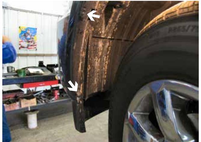
3. Just forward of the front tires, in the wheel well, remove 2 Phillips screws.
