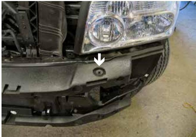
8. Remove the 3 push pins on top of the Styrofoam, pull forward and set the Styrofoam aside. (The driver's side is shown.)
